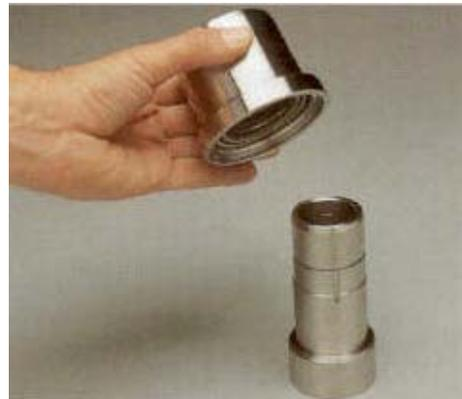
4. Slide the rotary seal housing over the shaft sleeve (24). Carefully push the sleeve past the slide rings and the lip seal. The rotary seal housing must fit completely over the shaft sleeve. Install the shaft o-ring (20) into the groove in the shaft sleeve.
