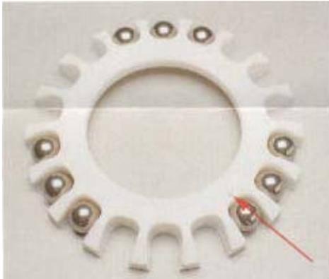
10. Place the balls (40A) into the slots of the ball retainer (40). For smooth operation, the balls must be symmetrically placed. Please note the small hole on the face of the ball retainer. This hole will fit over the spring pin (34B) in the ball housing (34).
