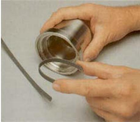
1. Place the slide rings (24A & 24B) into the bore of the rotary seal housing (24). The shortest slide ring goes into the rear of the housing.
