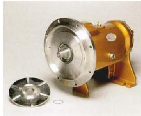
10. Slide the shaft sleeve o-ring (18) onto the shaft and install the expeller. Be sure the o-ring is seated into the groove on the shaft sleeve.
