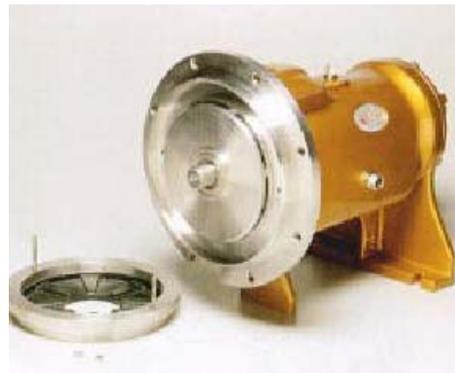
11. Install the seal housing gasket (30A) and case plate (15) to the frame. The studs (15A) go through the frame to secure with nuts (15B).
