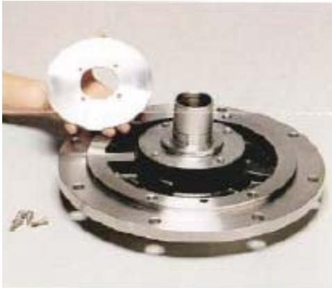
9. Attach the actuator (43) to the top of the rotary seal housing. The notch on the I.D. faces down. Be sure the drive screws (24C) and drive nuts (24D) are securely tightened, and use Loc-Tite® 261 or its equivalent on the threads.
