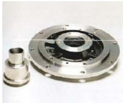
8. Slide the seal housing assembly over the shaft sleeve assembly, be careful not to damage the lips of the stationary seal.
