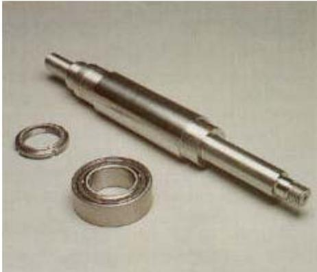
1. Install the outboard bearing (62B) and locknut (62C) onto the shaft (62). We recommend that a bearing heater be used when installing bearings to avoid damage to the races. Be sure the bearing seats against the shoulder of the shaft. If the pump is grease lubricated, hand pack the bearings with the appropriate grease (*reference Section 8*) after the bearings are seated on the shaft.
