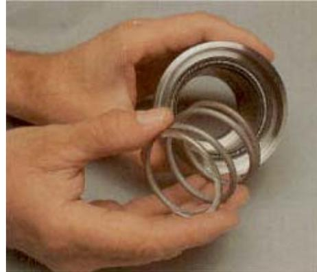
3. Insert the spring (42) into the bore of the rotary seal housing. Be careful not to damage the lip seal.
