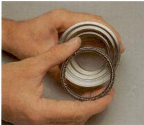
2. Insert the lip seal (25) into the rotary seal housing. Be sure the internal spring of the seal faces out. The seal must seat completely in the groove of the rotary seal housing.
