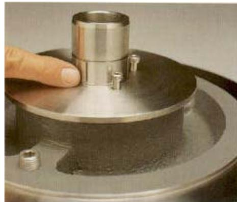
13. Slide the key (34C) into the slot on the shaft sleeve. You may need to push down and compress the seal assembly to fit the key into its slot.
