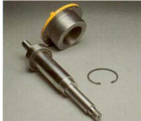
3. Slide the bearing carrier (72) onto outboard bearing and secure with retaining ring. Extreme duty bearings have a bearing plate that bolts to the bearing retainer instead of a retaining ring.
