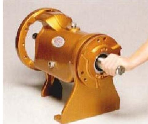
7. Install the bearing carrier o-ring (72A) into the groove of the bearing carrier. To avoid damage, lubricate the o-ring with light oil and slide the assembly into the frame. The word "top" on the carrier must face up. Attach the bearing carrier with three retaining bolts (75), jacking bolts (75), and jam nuts (72B). Clearance values and adjustment procedure follows the DryLock Seal assembly steps.
